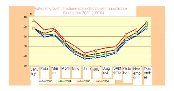
Thus it is necessary to notice, that, since July, 2006 because of favorable hydrological conditions on a number of the rivers of Russia, the increase takes place in monthly development of the electric power at HYDROELECTRIC POWER STATION. So on Angaro-Yeniseisk cascade in November, 2006 electric power development in comparison with November, 2005 has increased by 0,7 billion kW/h (9,7%), and as a whole on HPS on 1,4 billion kW/h (10,5 percent).
